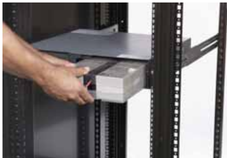
UPS models like the Eaton 9130 feature hot-swappable batteries for maximum uptime
